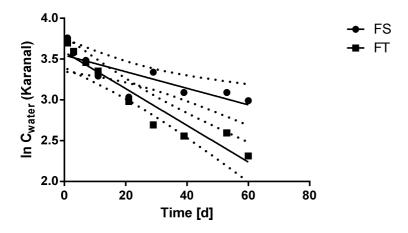
Figure 8. Semi-logarithmic plot of the residual concentrations of the substance in the test vessels (FT) and the residual concentrations in the sterile controls (FS), as a function of time
